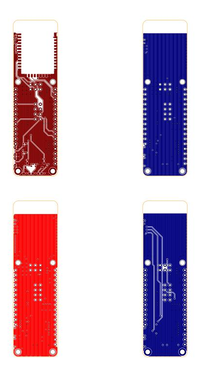
Figure 7: Top, bottom and internal layers
