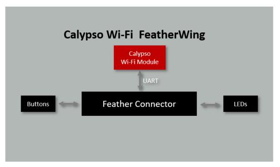
Figure 2: Block diagram - Calypso FeatherWing
